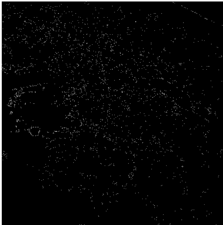
Figure 11. The difference image for the best transform evolved from the integer 2/6 . The much smaller number and reduced intensity of dots is indicative of substantially reduced MSE.
